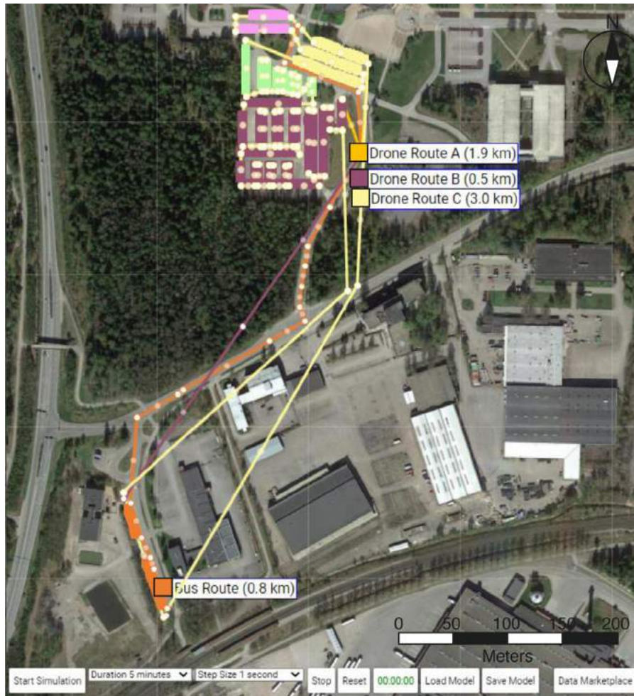
Fig. 7. A simulation model that comprises four routes, five observation targets groups and 455 observation targets for the parking spaces in parking areas A and B in the satellite view of the DMS tool.
