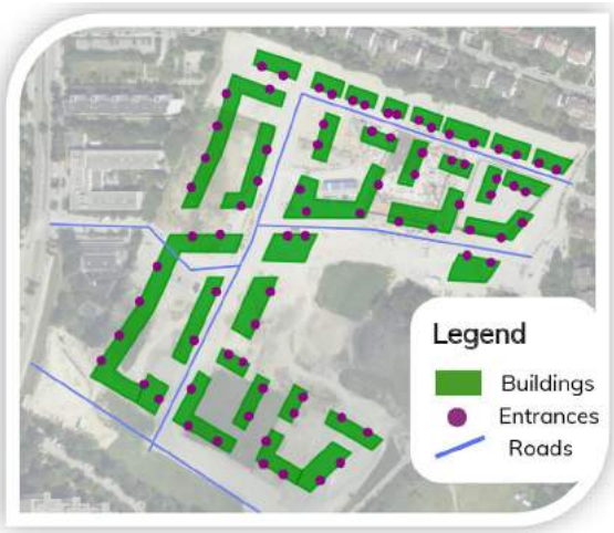
Fig. 15. Scenario with buildings uploaded from a building development plan and new road infrastructure.
