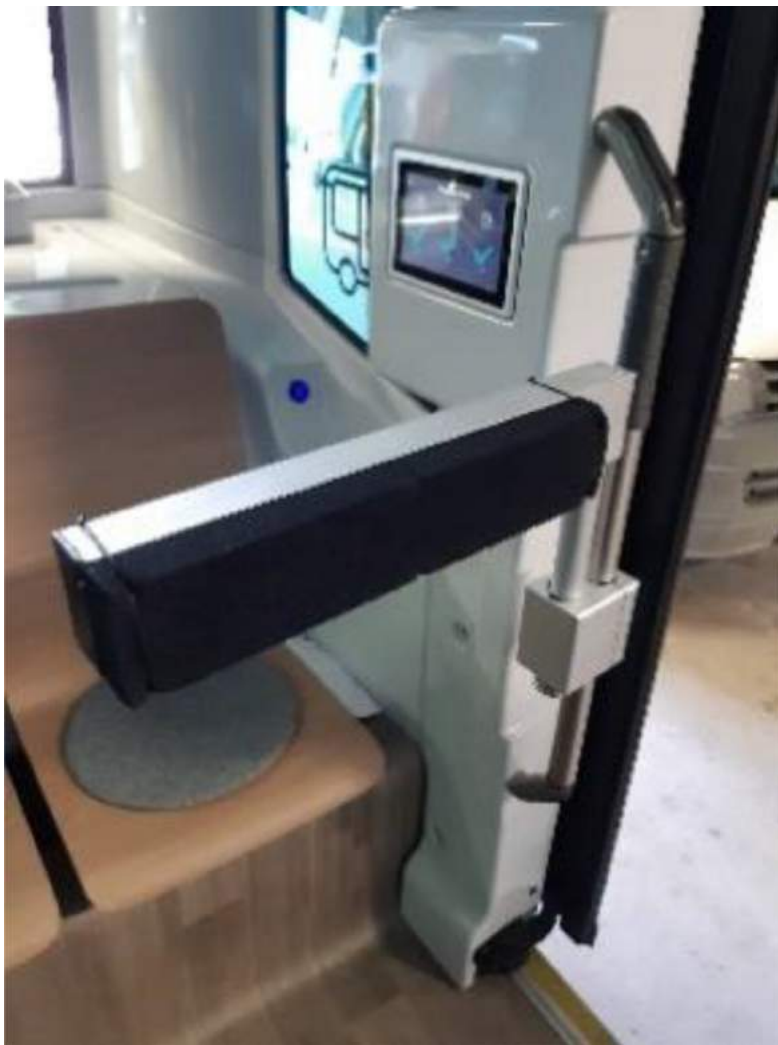
Fig. 9. Safety arm to support safety operators during ride, developed by VTI, Sweden.
