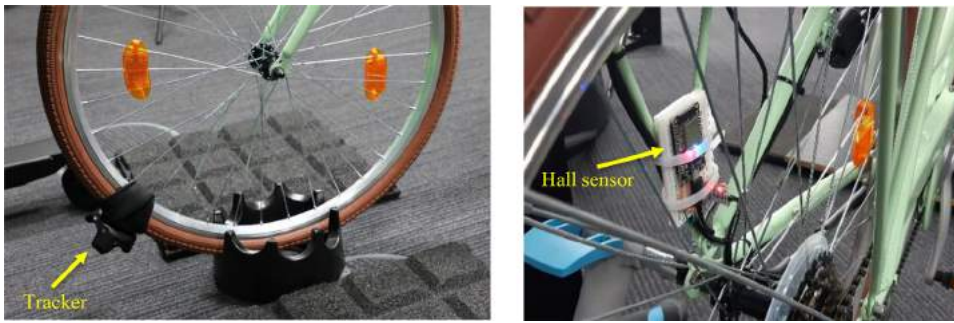
Fig. 3. Tracker at the front wheel (left) and Hall sensor at the rear wheel (right).
