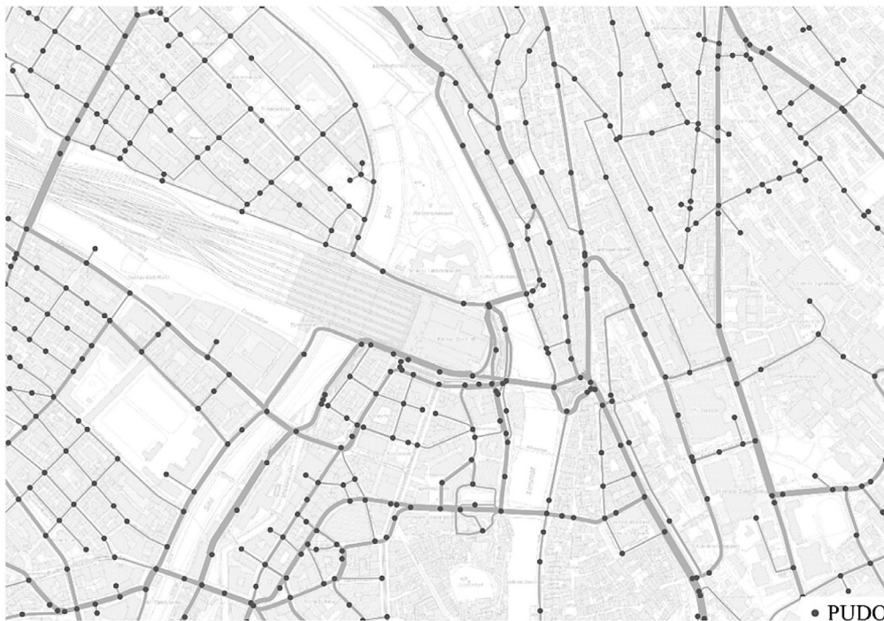
Fig. 2. Extract of the network model including the added PUDOs for determining the stopping points of SAEVs.
