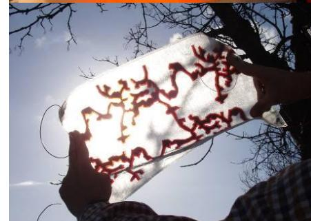
Risø DTU solar cell printed on textile. Screen print (fast)
